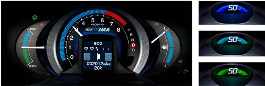
Fig. 1 Honda Insight hybrid dashboard and speedometer
