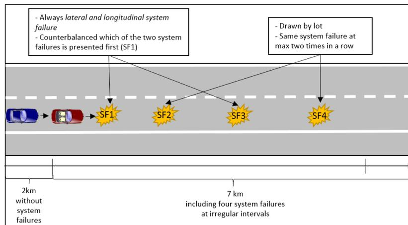
**Figure 1 – Types and order of system failures during each test drive. SF = system failures (adapted from Rauh et al., submitted for publication).**
