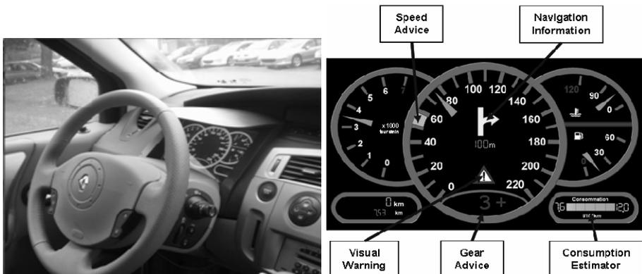
Fig.5. GERICO instrument cluster view
