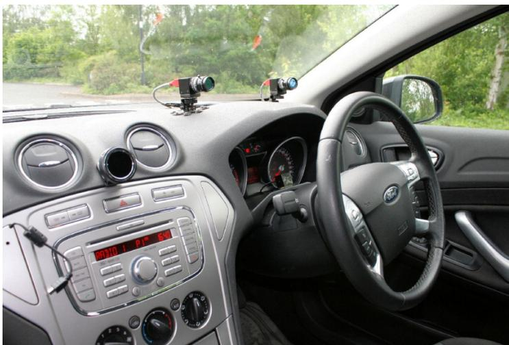
**Figure 1 Instrumented vehicle with eye-tracker cameras.**
