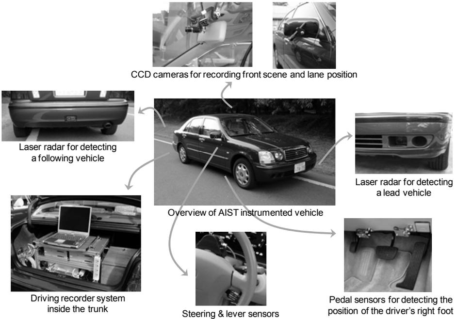
**Fig. 2 AIST instrumented vehicle**
