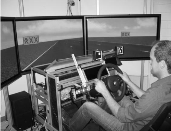
**Fig. 2: ALCT setup in a driving simulation environment**
